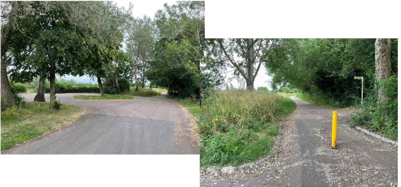
Figure 14: Photos of Examples of a preserved rural lane converted to walking and cycling route through 'stopping up' of vehicular traffic (left) and use of bollards/vehicular access controls (right)
